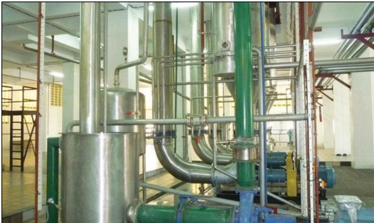
Picture 3 Kensalt 3-effect, 5 tph vacuum salt refining plant in Mombasa
